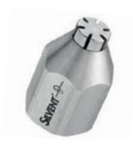
**SILVENT 700 M:** specially made entirely of stainless steel with aerodynamic slots to allow optimal utilisation of compressed air while keeping the noise level to a minimum. Hexagonal design fits a 14 mm (0.55") wrench.
